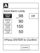
5. Press **ENTER** key on Programming Module to confirm.
