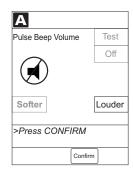
To increase volume, press Louder soft key until desired volume level is attained. To test volume level (when not attached to patient), press Test soft key. To turn off pulse beep entirely, press Off soft key.
