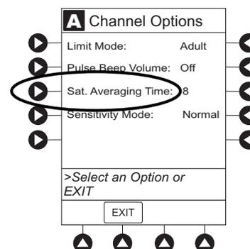
2. To change **Saturation Averaging Time**, press applicable soft key. Selectable options are **2, 4, 8, 10, 12, 14,** and **16** seconds.
