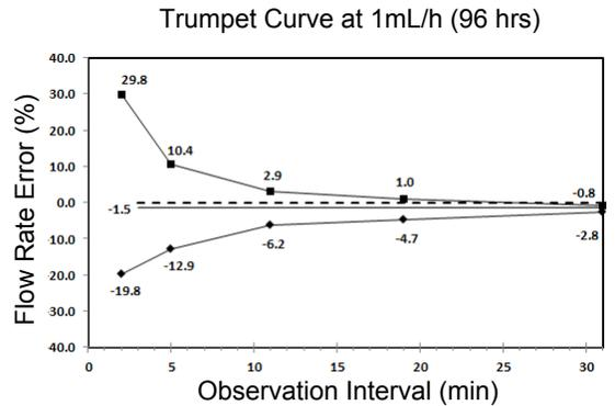
**NOTE:** The plot range has been increased to  $\pm 100\%$  to allow visualization of the graph.
