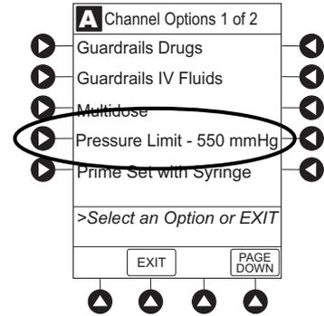
5. To enter a new pressure limit value, press **Change Value** soft key.<sup>①</sup>
