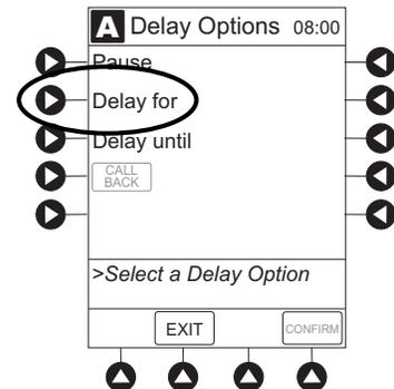
3. To enter number of minutes (up to 120) infusion is to be delayed for, use numeric data entry keys.
