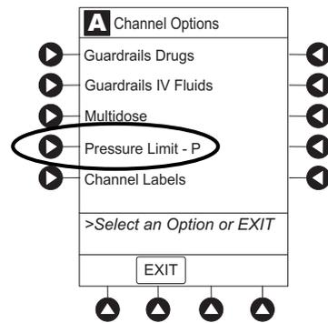
4. Press either **Pump** or **Selectable** pressure soft key. If **Selectable** is pressed, continue with next step; otherwise, proceed to last step.
