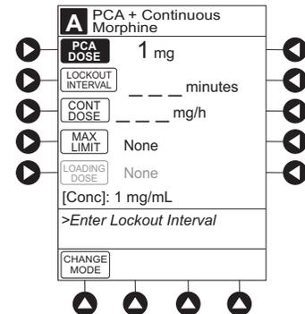
4. To enter lockout interval, press **LOCKOUT INTERVAL** soft key and use numeric data entry keys.
