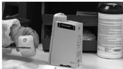
5. Clean both IUIs with the dedicated IUI cleaning brush. To avoid accidentally depositing fluid on the connectors, DO NOT use any spray cleaners anywhere near the IUI connectors.
