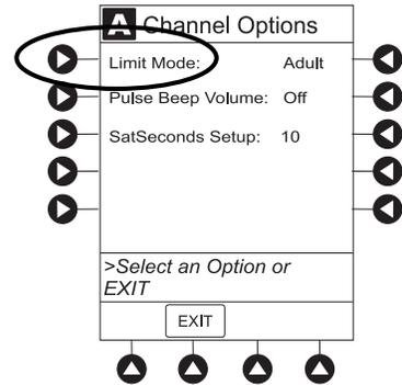
2. To change **Limit Mode Setup**, press applicable soft key.
