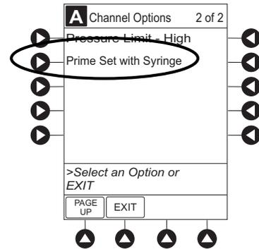
3. Press and hold **PRIME** soft key until fluid flows and priming of syringe administration set is complete.
